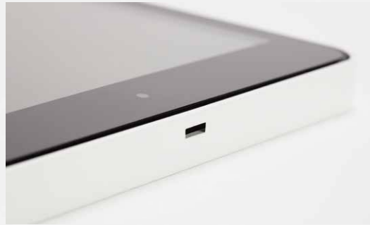
opening for the microphone
